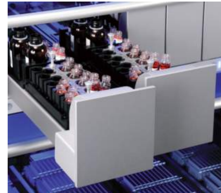
2 reagent drawers with a total capacity of 54 liquid reagents.
