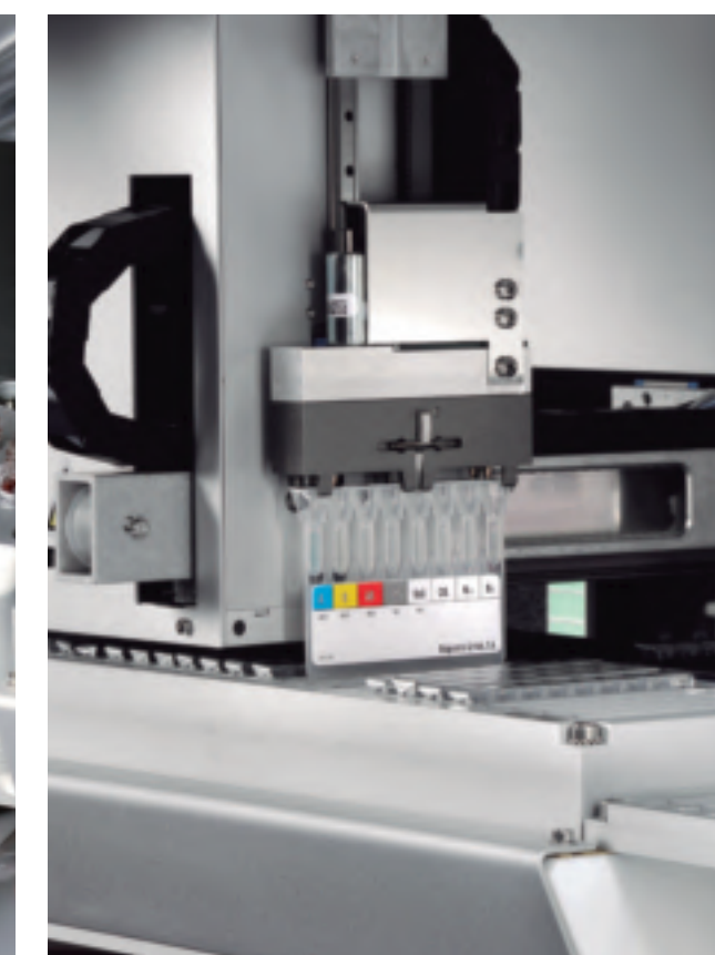
Working table and incubator with two independent areas for 37°C and room temperature incubations
